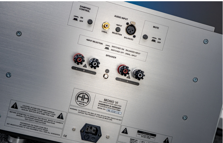
The back of the Mono VI: It offers two pairs of terminals on the output side. They are labelled “A” and “B”. However, both outputs are equivalent. This dual design means that transducers can be connected using the bi-wiring method. The pole terminals are superb models from the nextgen range made by WBT. They have a minimal metal content in favour of maximum sound neutrality. They also come with a torque indicator: This ensures optimum contact pressure when using connectorless cables or cables assembled with shoes. The use of bare stranded wire is trickier, as the terminal pins have no openings for the conductor entry. Cables with shoes or banana plugs are therefore the first choice. If the cable also has a separate strand for the shielding, the Mono VI even offers a separate earthing contact for this purpose.
