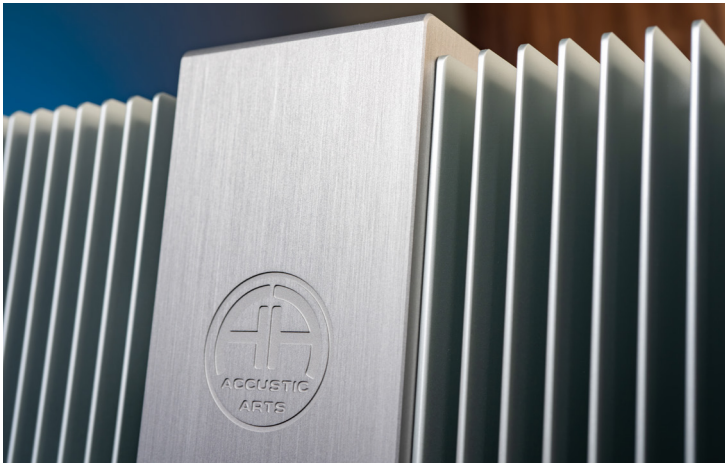
The ribbed areas serving as heat sinks are now even larger and thus promote heat dissipation. The amplifier's power transistors are in direct contact with these fins, which are milled from solid material, via a thick cooling plate on the inside. A new feature is the central subdivision of the ribbed series by a quasi-enclosing aluminium band with an engraved logo. The Mono VI thus benefits from a design feature that already characterises all current pre-amplifiers and integrated amplifiers in the Reference series.
